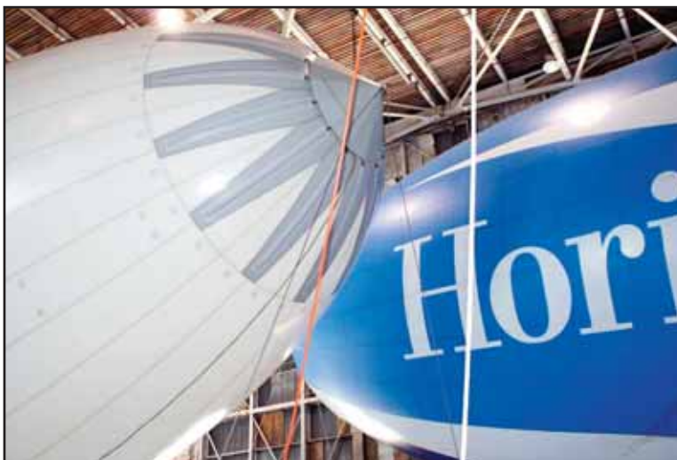
The A60+ is clear without the advertising decals. The decals are computer generated and printed and weigh 200 pounds.
