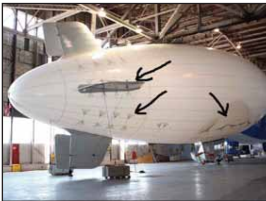
Interestingly, sheer patches hold the gondola under the envelope (body). Each one of these patches can hold 10,000 pounds.
